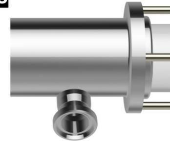
CIP connection built into pump body. This option enables insertion of washing fluid in the pump body to clean hygienic pumps in the best way possible. Manufactured tangential to the body, it avoids stagnation and enables efficient drainage of the fluids.
